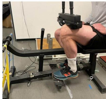
Figure 2. Calf muscle device isometric strength measurement
